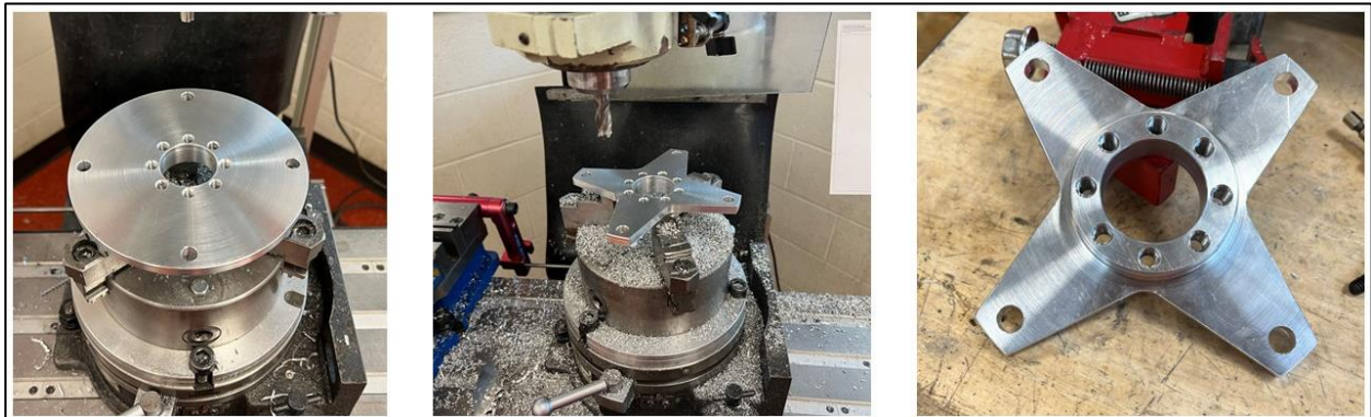
Figure 28: The leftmost image is the turned workpiece on the mill rotary table after all holes have been drilled, tapped, and reamed. The centre image showcases material removal using a rotary table to create the four spokes. The rightmost image shows the completed 7075-T6 hub adaptor.
