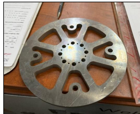
Figure 27: Finished 7075-T6 strain plate after two manufacturing processes; waterjet and CNC milling.
