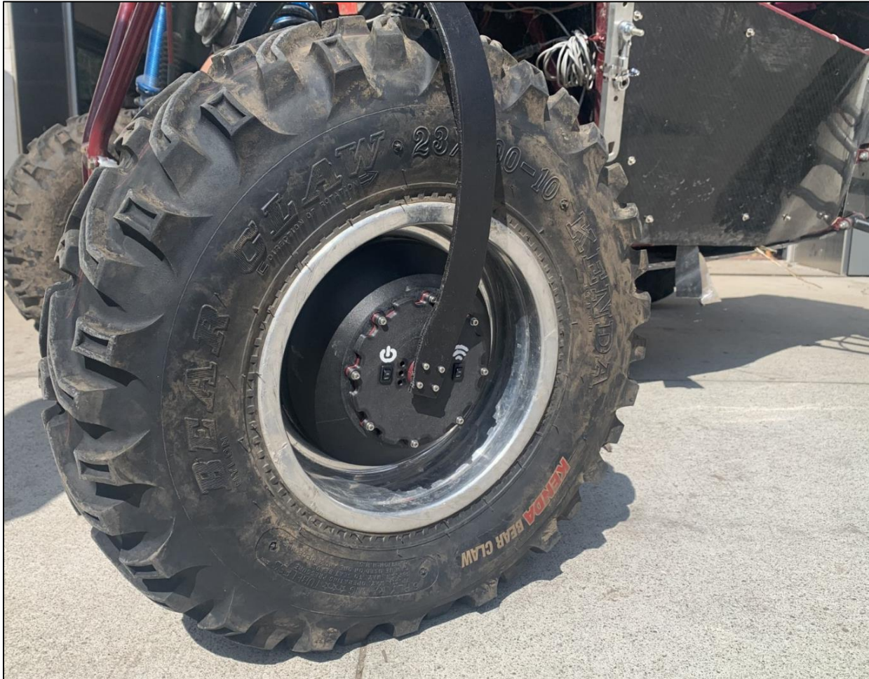
Figure 40: View of the WFT mounted to the wheel of the car, showing the new 3D printed cover, added to protect the WFT's DAQ system from any dirt or debris while the car is driving.
